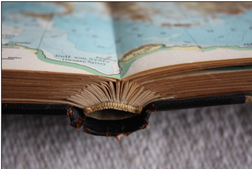
A 1948 School Atlas with hinged four page signatures-techniques used to achieve an uninterrupted panoramic view. Photo by Werner Rebsamen
